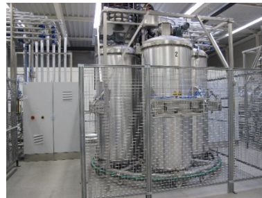
Infrared drying and cooling system
